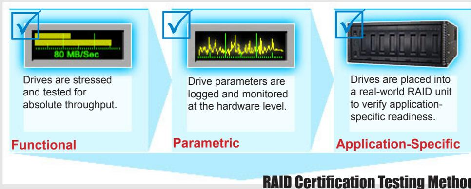
The third, and most crucial feature of DNF's certification procedure is application testing. Taken individually, drives will often behave within the manufacturer's specifications, but variations in the building process can cause problems in RAID situations. As data is striped across a high-performance RAID array, each drive accepts an exact
